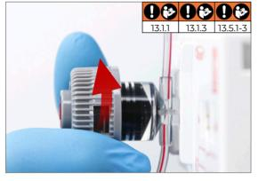
Completely open reservoir slowly by turning anticlockwise.
