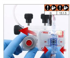
When filling the reservoir, open it slowly <sup>3</sup>/<sub>4</sub> of a turn (270°) anticlockwise and then close again.
