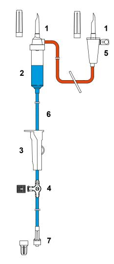
**5.** The hydrophobic 0.2 micron filter integrated in the spike ensures sterile ventilation and prevents aerosols.
